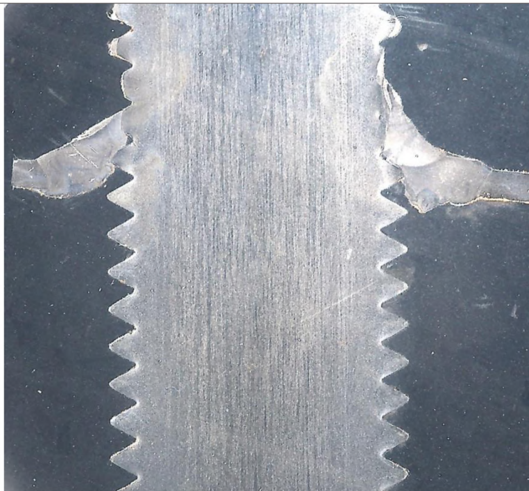
Figure 23: Section through welded region showing large heat affected zone (HAZ) and destruction of threads due to weld heat input
