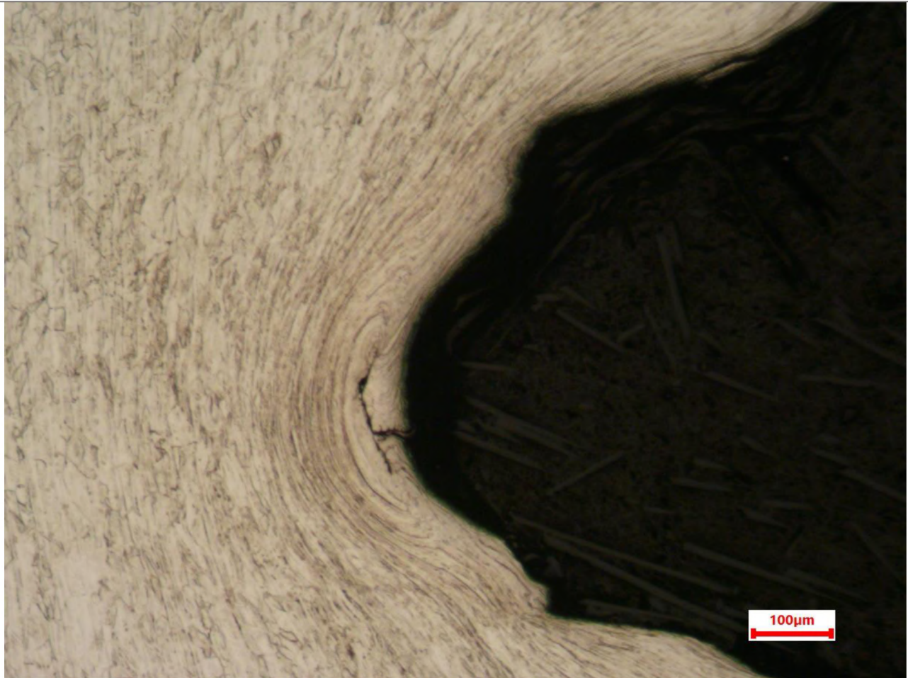
Figure 26: Microphotograph showing cracking at the thread root following the structural flow. Etchant: Kallings No 2 Magnification: x100
