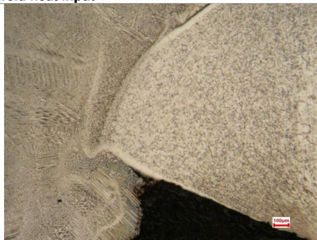
Figure 23: Section through welded region showing large heat affected zone (HAZ) and destruction of threads due to weld heat input
