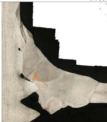
Figure 23: Section through welded region showing large heat affected zone (HAZ) and destruction of threads due to weld heat input
