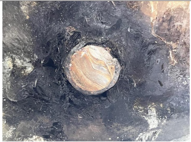
Figure 4: Fracture face of threaded bar, higher magnification showing fatigue beach marks
