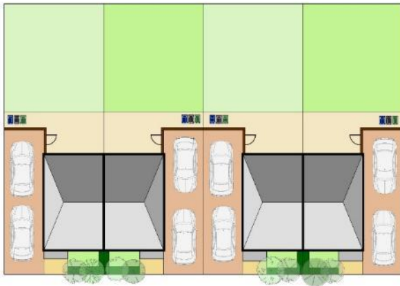
Side driveway parking, reducing car dominance in the street scene.
