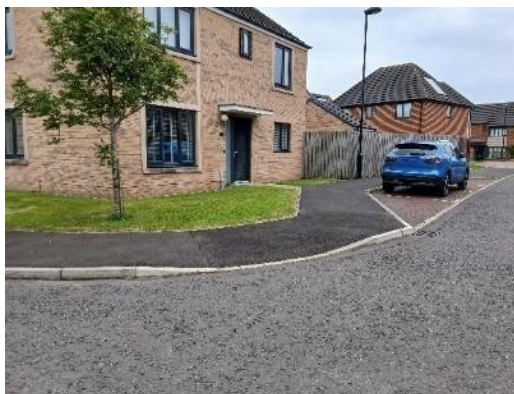
Dropped kerb at street corner providing step-free access.
