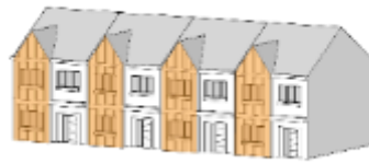
Repeating projecting bay windows adding visual interest.
