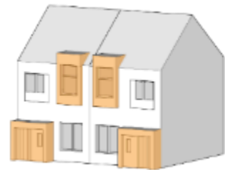
Projecting entrances and upper-level window features.
