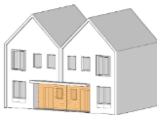
Projecting canopy over recessed entrance
