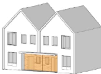
Projecting canopy over recessed entrance
