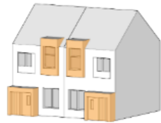
Projecting entrances and upper-level window features.
